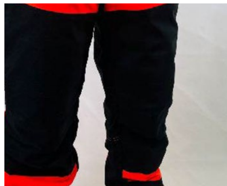
Special spacer fabrics provide impact protection that can cushion the im-pact of a wild boar attack by up to 20 per cent. Stab and cut protection are also guaranteed. © 2026 STFI
