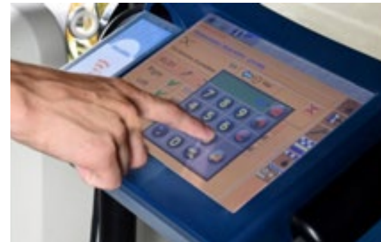
Electronic Setting of Shed Crossing (AKM) © Picanol
