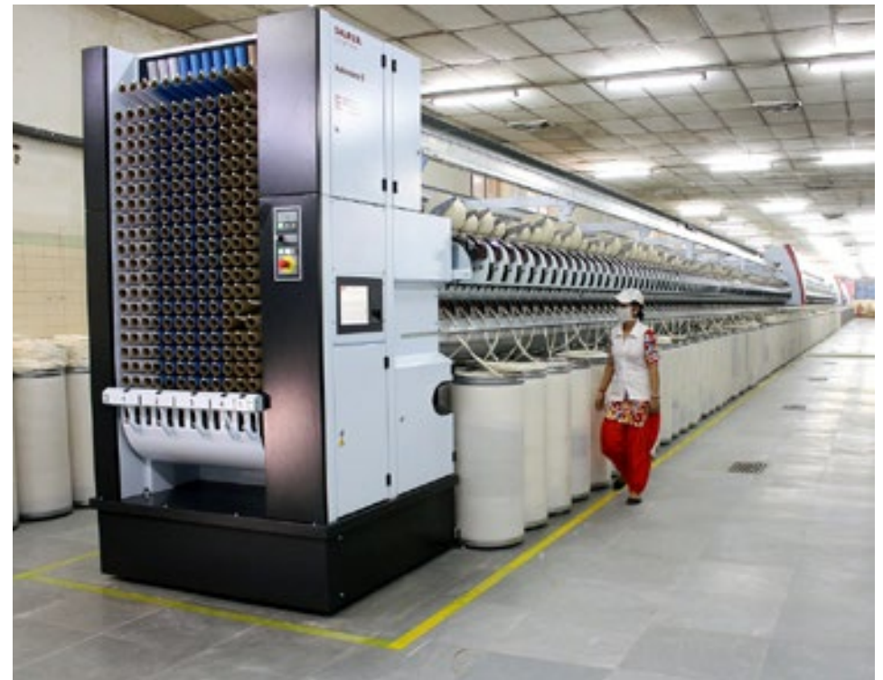
The new Autocoro 9 with 720 spinning positions at T.C. Spinners © Saurer
