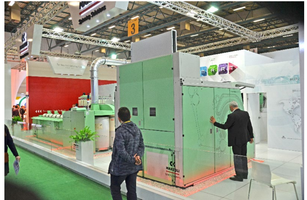
Marzoli decided to present an automatic combing machine from its wide range of machines for spinning preparation and spinning.
