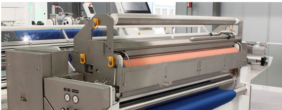
BRÜCKNER ECO-COAT minimum application coating unit for technical textiles © 2018 Brückner
