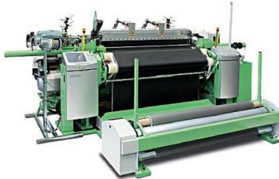
Rapier Weaving Machine P1, type PTS 8/S20 C © 2018 Lindauer DORNIER
