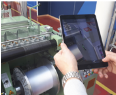
Figure 2: Augmented reality-based assistance system for maintenance and servicing © ITA
