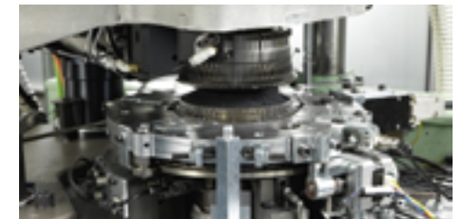
D4S toe-closing device: Automated knitting solution by Stäubli © 2021 Stäubli
