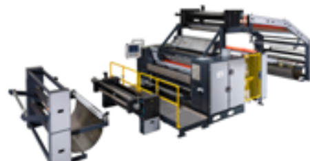
CAVIMELT – The rotogravure system for fabric lamination © 2021 SANTEXRIMAR
