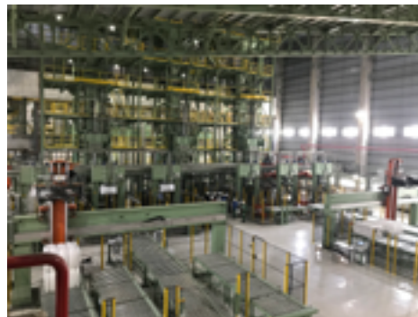
Autefa Solutions UNI-FORK System with 3 pre-presses and 6 main-presses © 2021 Autefa Solutions
