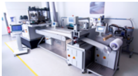
NIRI's new pilot-scale meltblown machine © NIRI
