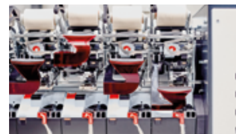
Equipped with SynchroPiecing, each AutoBD rotor-spinning machine can run up to 1 500 piecings per hour fully automatically, which means that there is hardly any dependency on staff availability © 2021 Saurer
