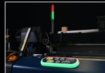
Connect generation - Smarte Signalleuchten © 2021 PICANOL
