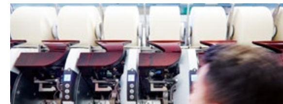
The light concept above the spinning positions enables an efficient operator guidance © 2021 Saurer
