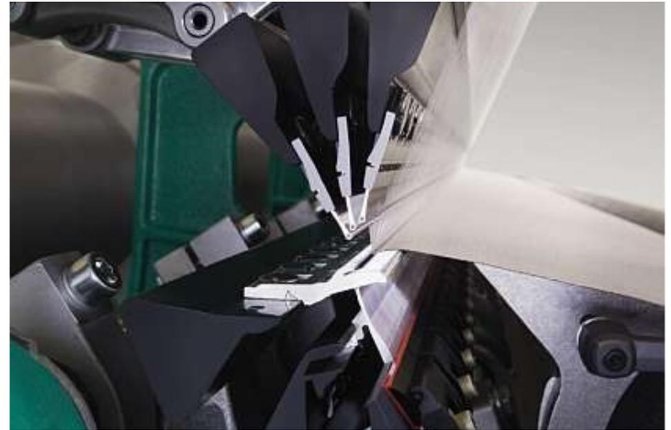
Karl Mayer warp knitting machine with components from CFRP
