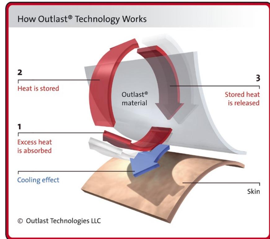
Outlast - How Outlast technology works
