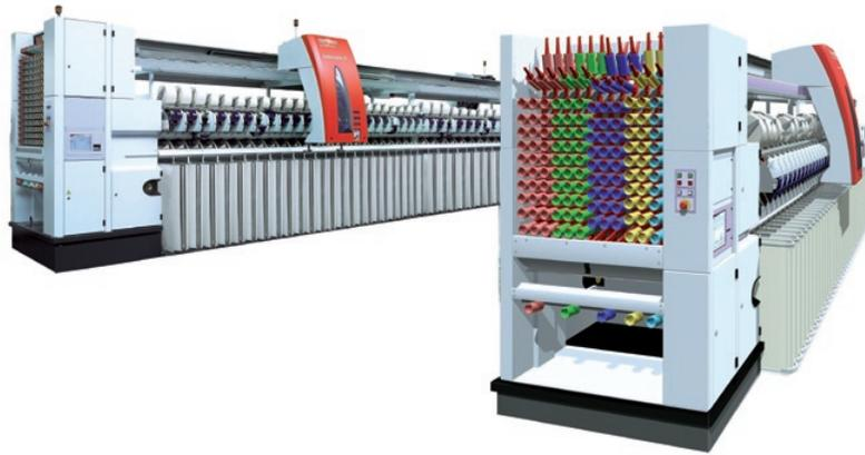
OERLIKON SCHLAFHORST - Rotor spinning machine Autocoro 8
