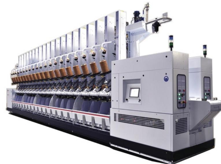
Volkmann Heat-SET integrates heat-setting in the cabling process
