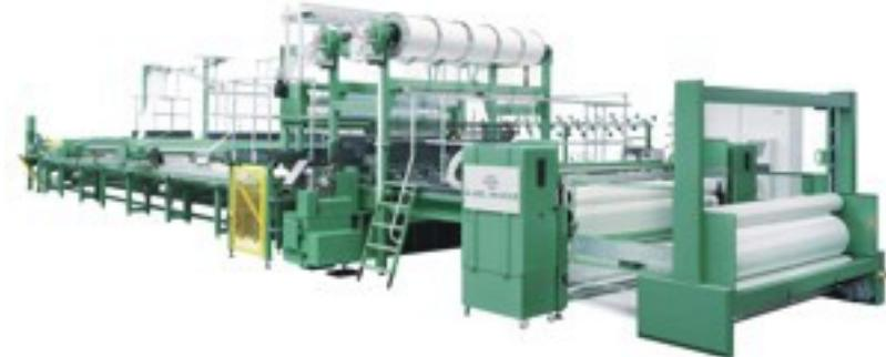
KARL MAYER - Multiaxial, High-tech knitting machine with several weft insertion systems for the production of multiaxial multiply and composite fabrics
