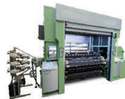
From wool to glass in one weaving workshop: The future-oriented encapsulated air-jet weaving machine brings different, individually controllable climate zones into the production workshop for the first time. © DORNIER
