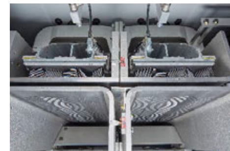
Needle arrangement "8000X" for a more even needlefelt surface © 2019 Dilo
