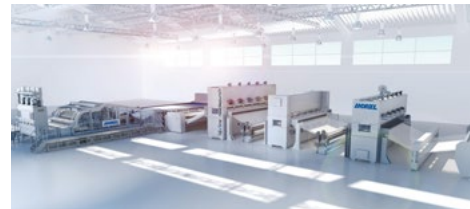
neXline needlepunch for the production of technical nonwovens dedicated to geotextile, filtration and automotive applications © ANDRITZ
