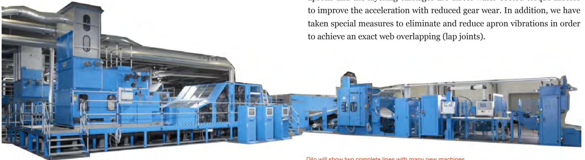
The universal model series “**VectorQuadroCard**” comprises variable components for all kinds of applications. Focus is laid on high throughput with good web quality. The “VQC” exhibited at the show with a working width of 3.2 m is designed for the geotextile sector.
