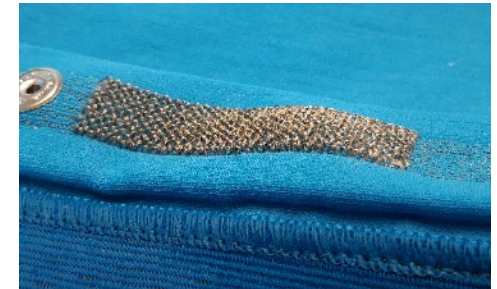
Warp-knitted sensors with optimised skin contact © 2022 KARL MAYER
