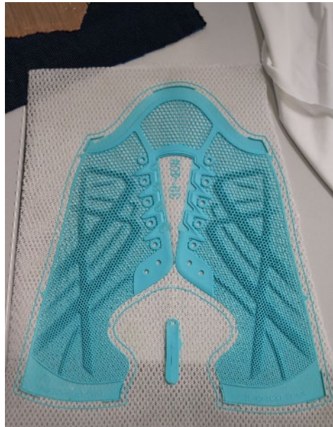
Warp-knitted footwear fabric with 3D-printed reinforcement structure © 2022 KARL MAYER
