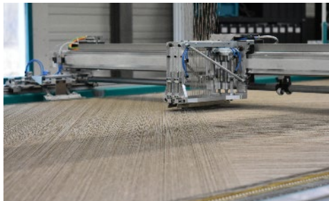
Processing of flax fibres on a multiaxial warp-knitting machine © 2022 KARL MAYER
