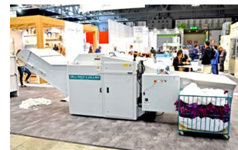
The recycling process starts with a Guillotine cutter © 2023 TexData International
