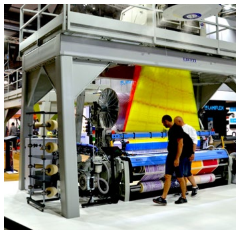
iteMa R9500 EVO terry weaving a terry towel - shedding by Bonas Jacquard Si6 6144 hooks © 2023 TexData International
