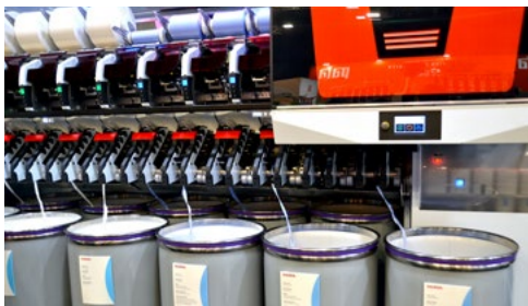
Autoairo air-spinning machine with autonomous spinning positions © 2023 TexData International
