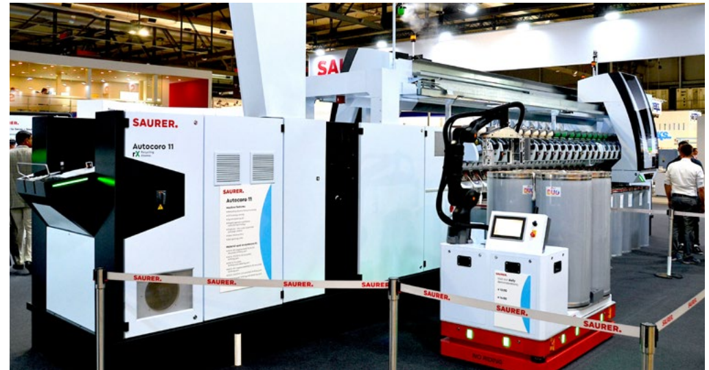
The new Autocoro 11 rotor-spinning machine for producing yarns from recycled fibres © 2023 TexData International
