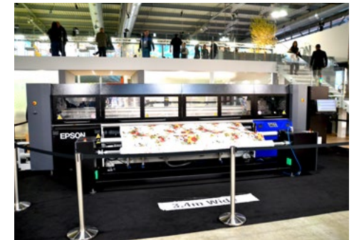
Epson Monna Lisa ML-32000 340 offers double-sided printing up to 340cm © 2023 TexData International
