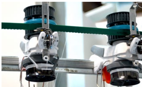
The cameras for the defect detection are built into the machine © 2023 TexData International
