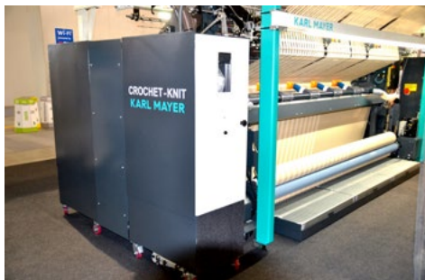
RSJFS 4/1 EL – CROCHET-KNIT machine © 2023 TexData International
