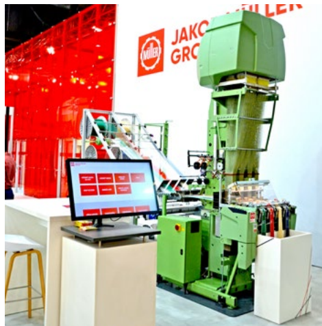
Electronically controlled Jacquard needle weaving loom NFMJ 53 4/66 © 2023 TexData International
