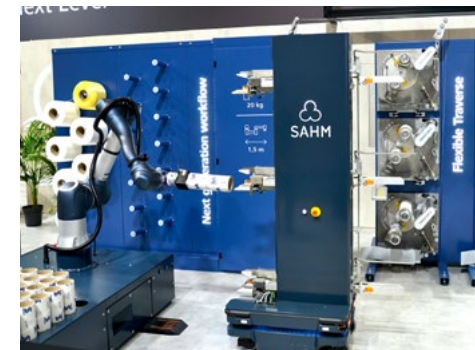
Bobbin change with the robot for the Twinstar II © 2023 TexData International
