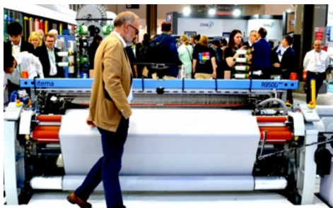
R9500 EVO weaving a nautical sails reinforcement © 2023 TexData International
