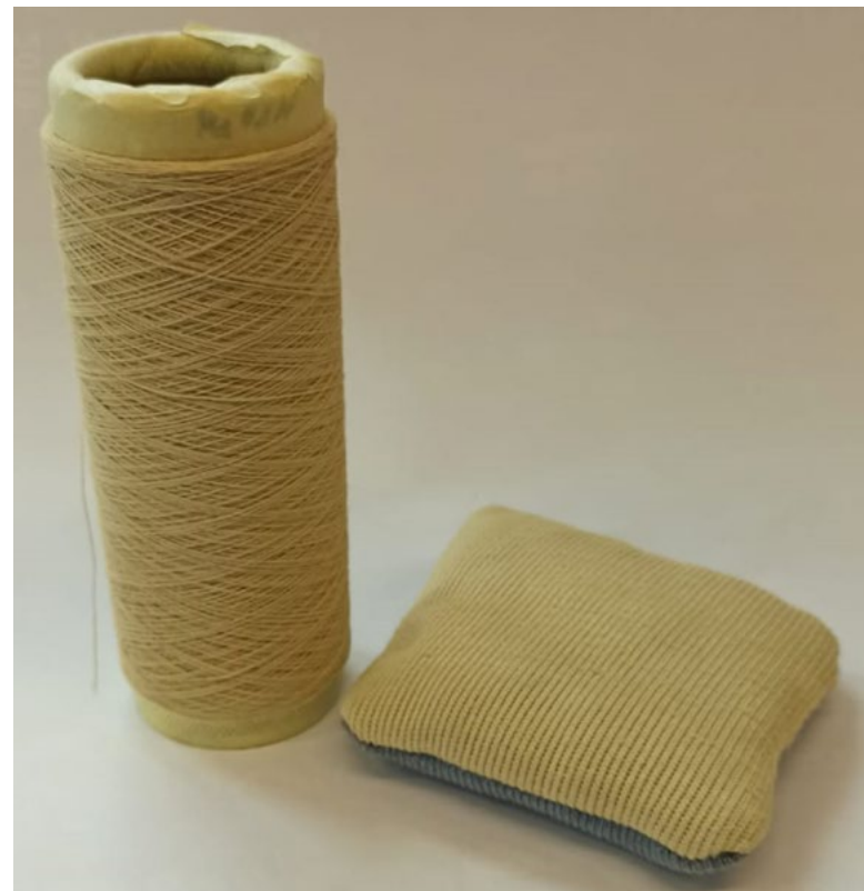
Fig. 1 - Staple fibre yarn and demonstrator knit of RePAN fibres. © ITA
