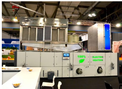
100% electric stenter shown by ICOMATEX © 2023 TexData International
