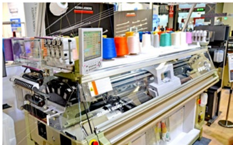
SHIMA SEIKI's SWG-XR® flagship WHOLEGARMENT® knitting machine © 2023 TexData International
