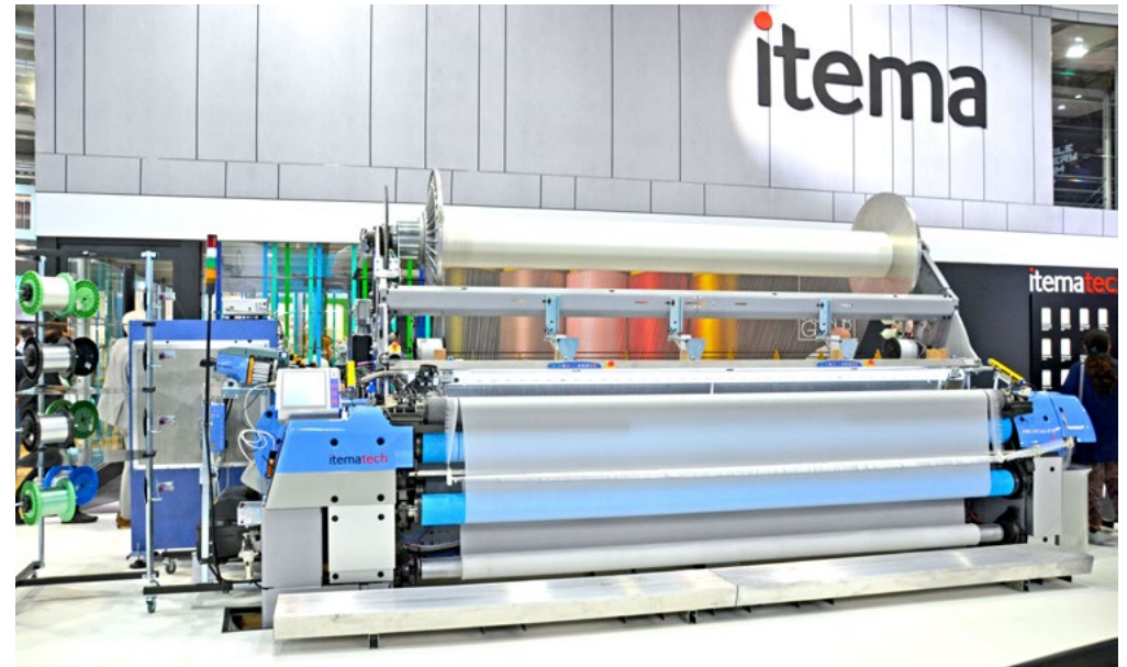
itematech showed the Hercules machine in 3800mm weaving a heavy filter fabric © 2023 TexData International
