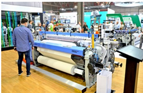
Also on display was the new A9500 EVO weaving a bottom weight from combed cotton © 2023 TexData International
