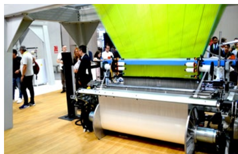
R9500 EVO in 1900 mm weaving a tapestry - shedding by Stäubli Jacquard LXXL 20480 hooks © 2023 TexData International
