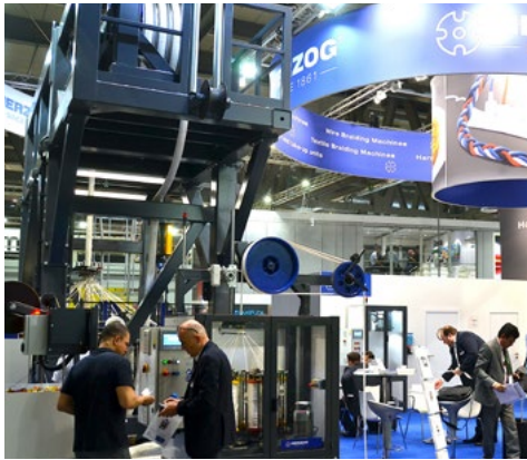
Herzog rope-braiding machine SE 1/12-266 and SE 1/32-432 in the background © 2023 TexData International
