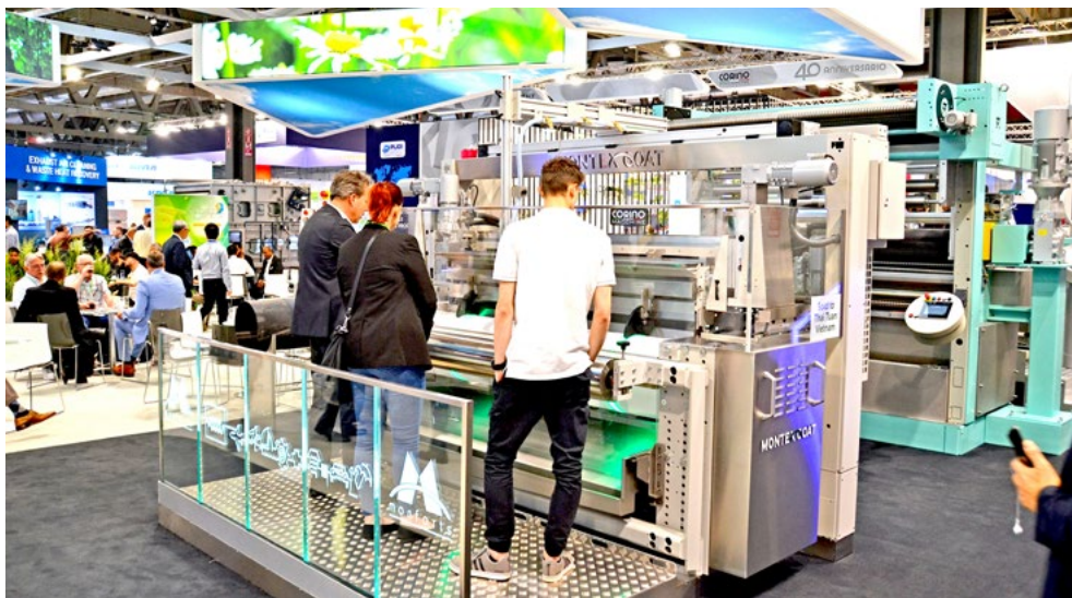
The Montex@Coat coating machine on display was equipped with a number of new features including automatic edge limiters for immediately adapting to new coating widths. © 2023 TexData International
