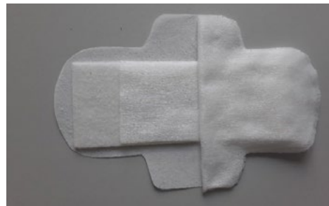
Nonwoven construction developed at STFI paves the way to reusable use for bio-based hygiene products © 2023 STFI
