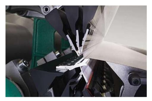
Karl Mayer warp knitting machine with components from CFRP
