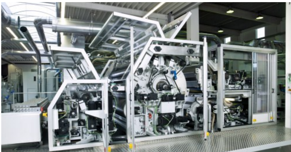
Trützschler 普梳EK150
