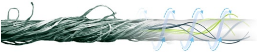
Fig. 3: Structure of the air jet yarn - Source: Herrmann Buehler / Povel
