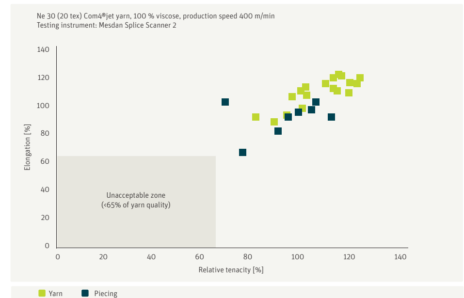
Fig. 5: Yarn-like piecing quality: the piecing has almost the same strength as the yarn without visible differentiation - Source: Rieter
