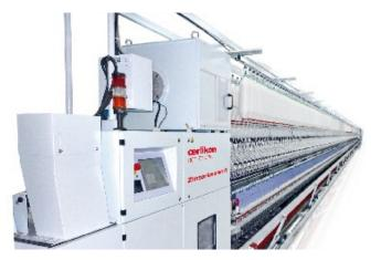
OERLIKON - The new Zinser Impact 71 ring spinning machine
