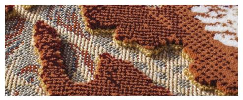
Filling effects on cut-loop carpet made on VAN DE WIELE carpet machine
