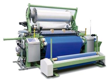
DORNIER - Rapier Weaving Machine P1 for the manufacturing of technical textiles
