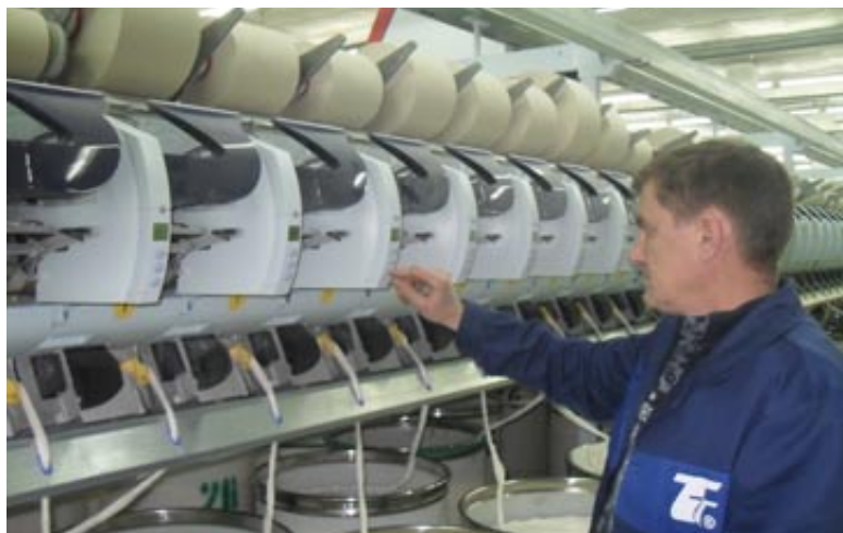
Autonomous individual spinning positions facilitate huge productivity increases of 18% and more
