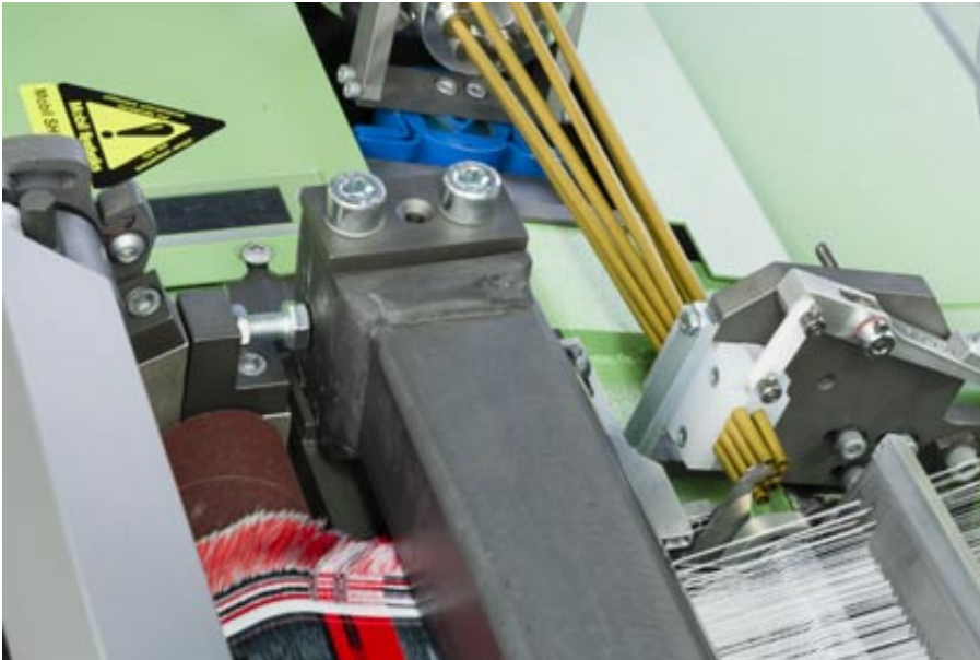
The main nozzles, which are designed for up to eight weft colours
