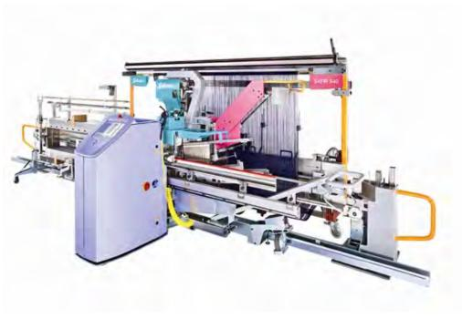
The new Stäubli SAFIR S40 drawing-in machine is an important step for automation in weaving preparation
