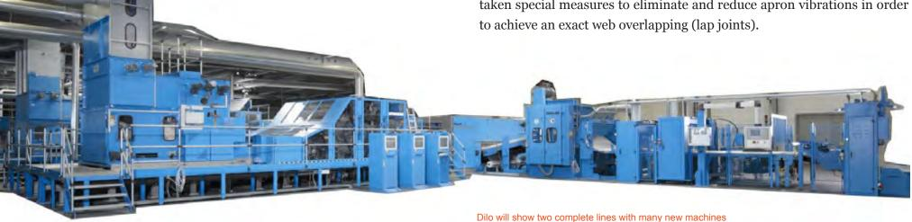
Furthermore, they have installed a "web guiding system" (FLS) to avoid wrinkles for example at the speed change of the upper carriage. The web infeed width is 3.2 m, the layering width is 7.0 m.
