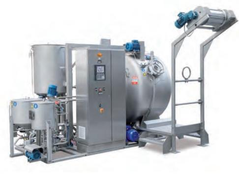
Other innovations are the soft-TRD SIII, which combines the perfect running conditions of the famous soft TRD SII with the latest short liquor ratio technology and the MPS-G which is the new, multi-functional supply system for chemicals, solids and dyes.
