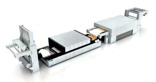
The Archer® print bar has been designed to retract fully for easy maintenance. Heads can be purged in narrow segments and a faulty head can be replaced by users in less than an hour, with no need for manual alignment – simply software-based registration. The heads are manufactured by a MEMS process, which means they are less liable to degradation and can be refurbished.
