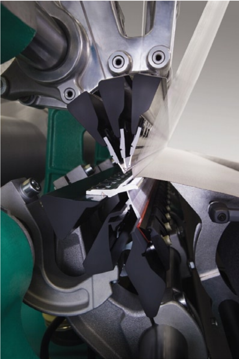
Karl Mayer: Cross-section view of a knitting place with CFRP bars
