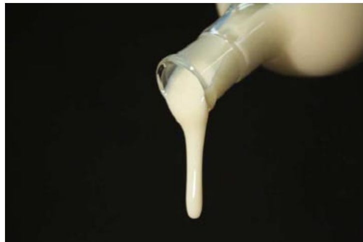
Ceramic textile pulp for the manufacture of corundum fibres
