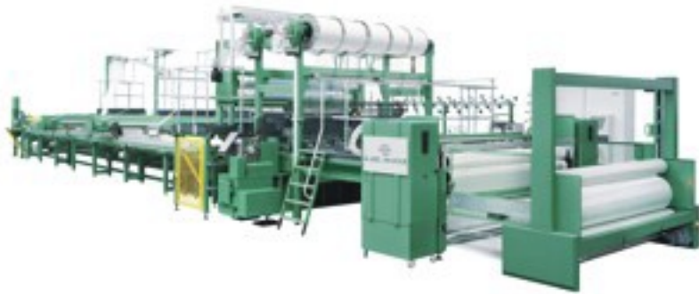
KARL MAYER - Multiaxial, High-tech knitting machine with several weft insertion systems for the production of multi-axial multiply and composite fabrics
